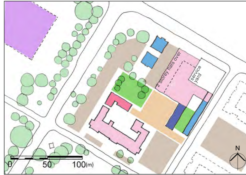
Option 1 - the supermarket is located with a frontage and service yard on Alison's Road, so as to create a public space between it and the Headquarters building.
