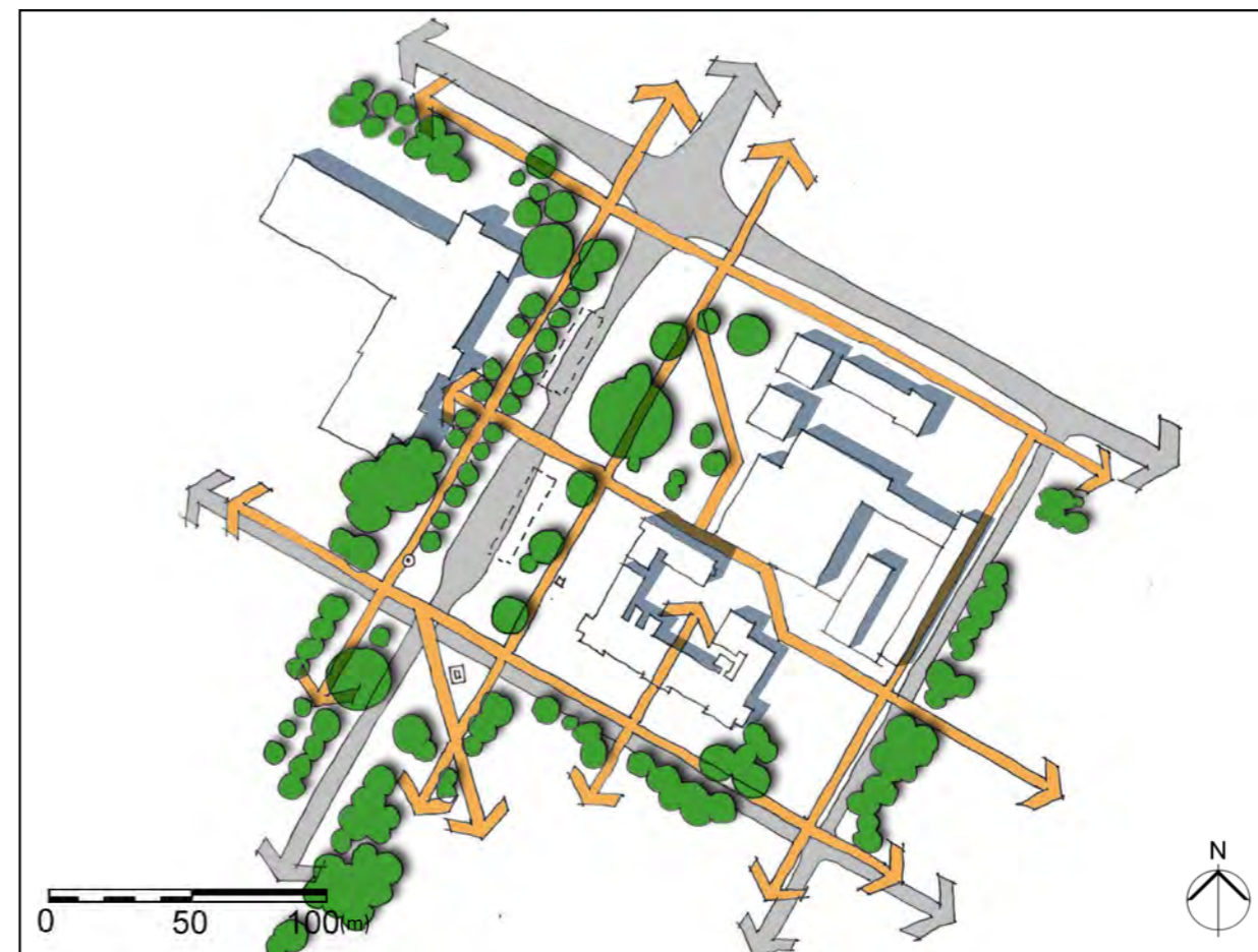
Sketch showing the principal pedestrian routes and desire lines around the Neighbourhood Centre
