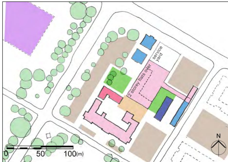
Option 3 - the supermarket is brought closer to the Headquarters building, creating a tighter and more defined public space between them.
