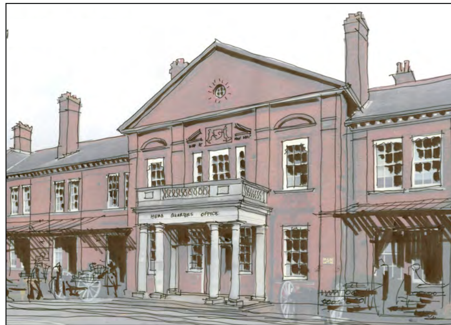
Sketch to explore the possibility of creating shop-fronts on the south facade of the Headquarters building - the window openings would have their cills lowered to the ground, or they would be enlarged, or even fitted with awnings and signage to advertise their use as retail units.
