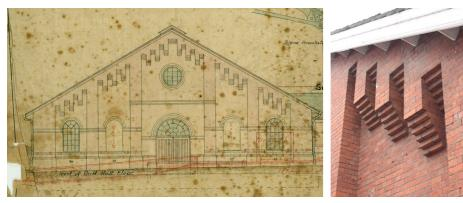
Original drawing for the southwest elevation of the Maida Gymnasium (above left) with a detail of its distinctive brickwork detailing (above right). The building is the only surviving remnant of the Maida Barracks, which were demolished in 1971.
